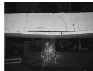
Failure mode for slab No.3, fibre rupture and partial debonding of mortar
